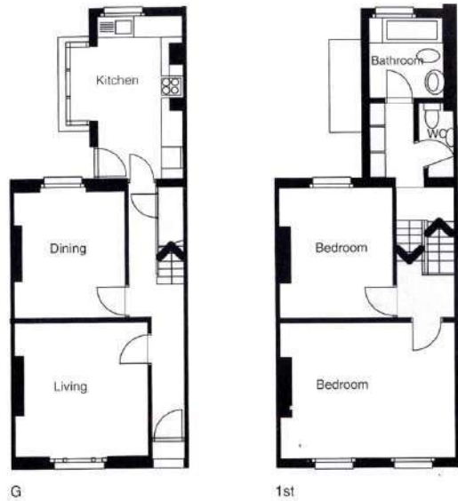
Plans of typical Victorian-terraced house
